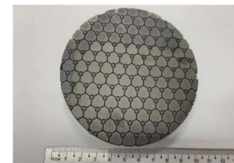
近零膨胀结构高纯氧化铝陶瓷盘 Ceramic Disc with Near-Zero Thermal Expansion Structure
