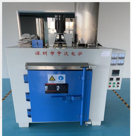
De-burning electric furnace equipment
